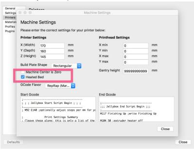
This will allow you to see the heated bed settings as 'Build Plate Temperature' in the 'Custom' tab under 'Material'
