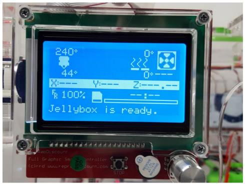
Using the controller, set the hotend temperature to 240\*C. (Press > Nozzle Temp > Nozzle > 240). Allow the hotend to reach 240\*C and wait one minute to allow all components to equalize in temperature. Tiny amounts of smoke are normal.
