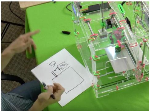
The X Homing offset tells the printer where the print area (build plate) effectively starts as the "home position" for x – the place at which X carriage hits the X endstop – puts the nozzle off the build plate. If the offset isn't set, under some conditions, the proximity sensor may cause problems trying to sense off the edge of the plate.
