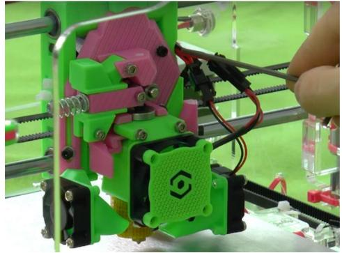
If you get misaligned layers, you should check the set screws in y and x pulleys first. Also make sure the extruder bolts are not loose.
