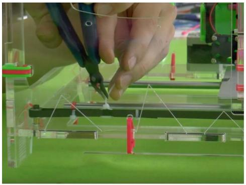
Try to put the Y assembly in the same position every time when adjusting the belts; this will help keep things consistent.
