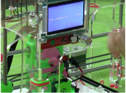
Push the knob to access the menu on the LCD display. Navigate to "Adjustments" and then "Fan Speed".
