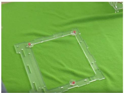
The etchings on the back piece should be on the side facing you; that is, the text should look mirrored.
