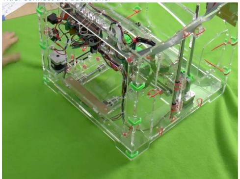
Use the six corner clips to attach the back panel to the box.
