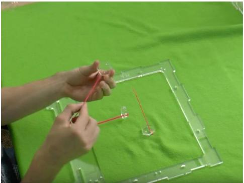
Thread a 6" zip tie through each hexagonal mount. (The toothy part of the zip tie should be facing the center point of the hexagonal piece.)
