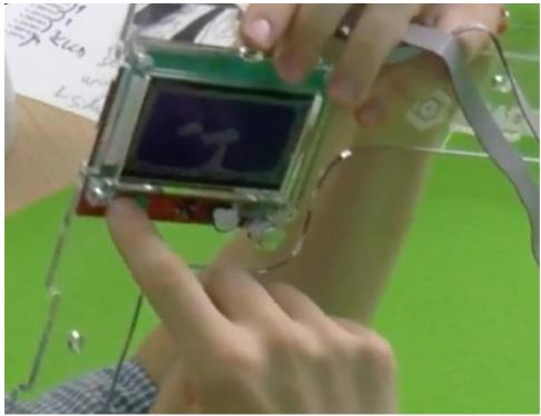
Attach the LCD controller to the front acrylic piece. Tighten screws in place with screwdriver or hex key. The 3mm spacer does not cover the lower left hole. Do not over-tighten this screw or you could damage your controller!
