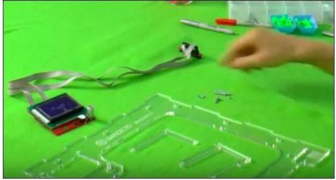
LCD display Front acrylic piece (it says IMADE3D JellyBox) Two acrylic spacers Four M3x25 flathead bolts Four M3 washers Four M3 locknuts
