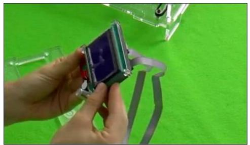
Align the 6mm spacer to the front of the controller.
