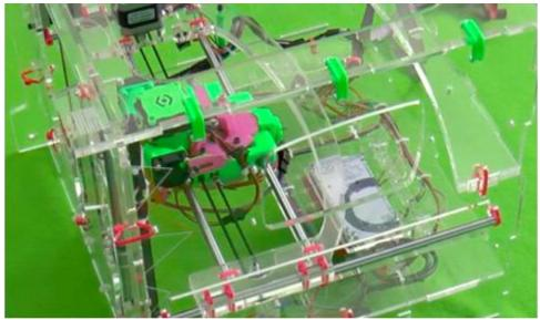
Fasten the front piece to the rest of the JellyBox using the green clips and 6" zip ties.
