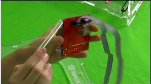
Sandwich the thin 3mm LCD spacer between the two layers of the controller. The one hole not covered by the spacer will be on bottom left.
