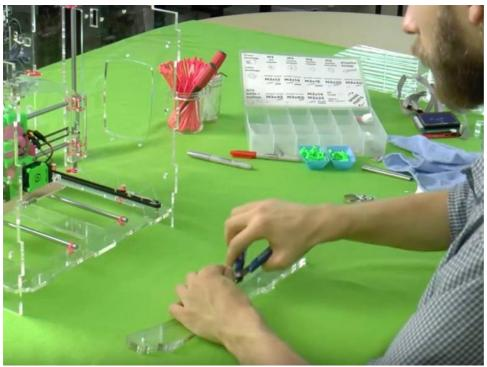
Use a 4" zip tie through the two central holes. Tighten the zip tie with vice grips. Cut the free end with side cutters.
