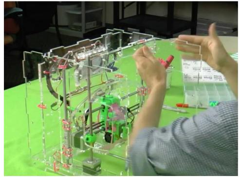
**Gently flex left and the right acrylic pieces** to put the brace into position. (See video if necessary!)
