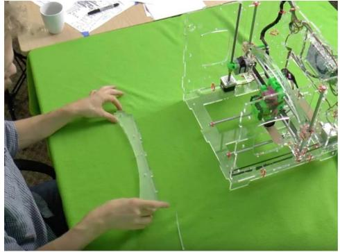
Place the front brace on top of the back brace.
