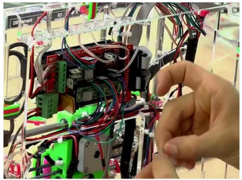
Peel off the sticky backing on a heat sink.
