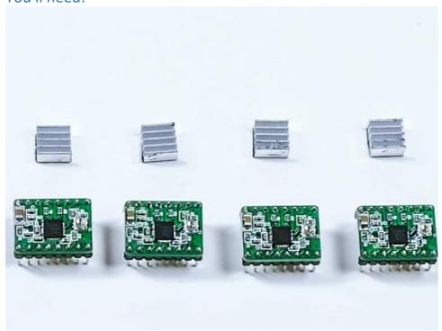
Small aluminum heat sinks (4) (The drivers are already on the RAMPS board.)
