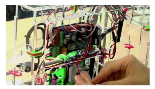
In this video, we add heatsinks to the motor drivers to keep them cooler. The heatsinks are not needed for JellyBox operation, but they prolong the component drivers' life expectancy.
