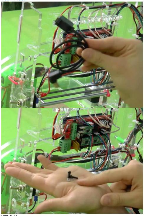
USB Cable M3x12 bolts (2) M3 serrated washers (2)
