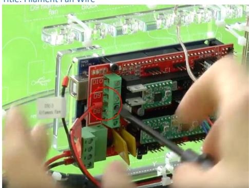
Connect the filament fan wire to D9 on the RAMPS board.
