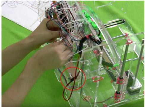
Connect the wire for the proximity sensor and hot end fan.
