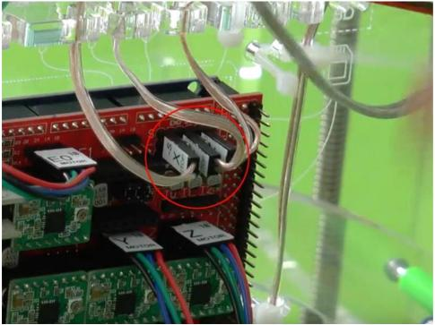
Connect the X and Z axis end stops next to the Y end stop connection. Make sure the labels are facing left.
