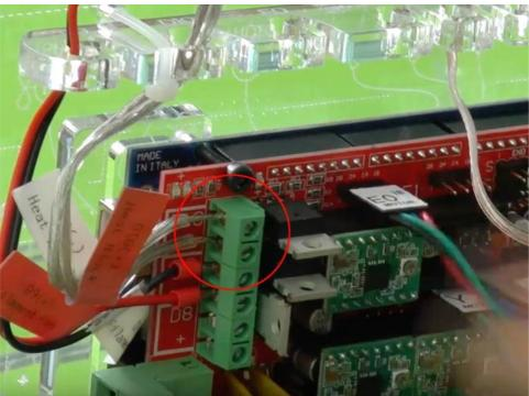
Connect the heat block wires to D10 on the RAMPS board.
