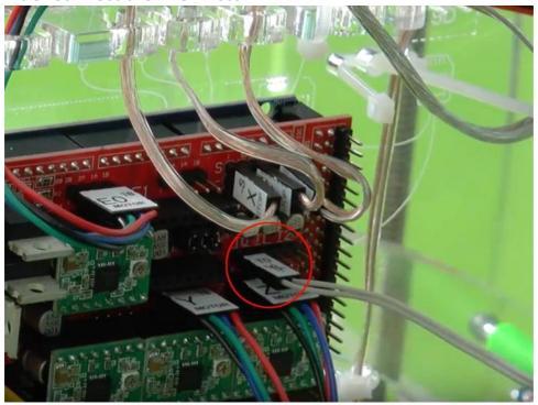
The thermistor wire connects to T0 with the label facing up.
