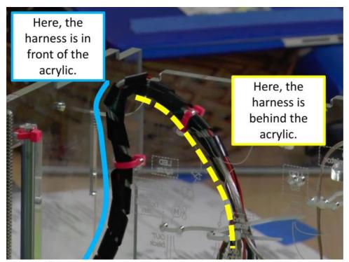
Use two 6" zip ties to secure the X wire harness to the inner back piece.
