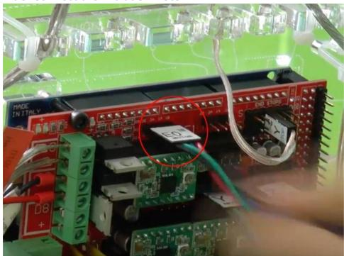
Connect the extruder motor to E0 on the Ramps Board. Make sure the label is facing upwards.
