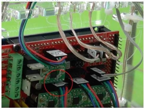
The X motor connects next to the Y and Z Motors. The label should be facing up.
