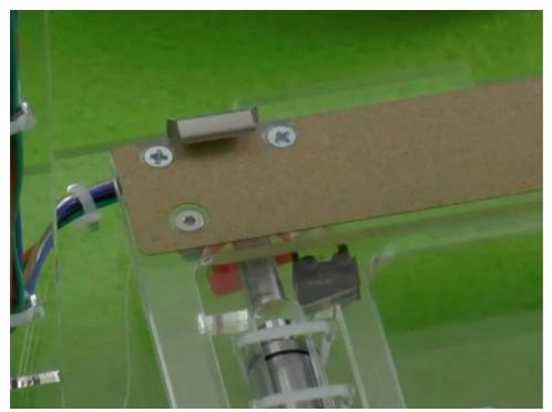
Make sure that the Y EndStop in the back of the Bottom piece gets engaged by one of the Y Assembly bearings!
