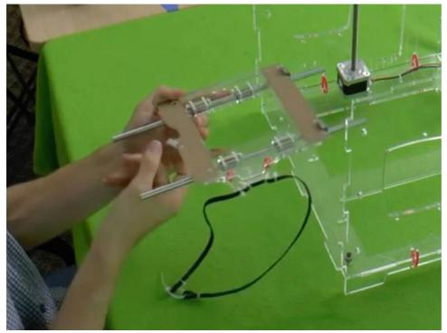
Thread the smooth rods through the bearings on the Y Assembly. Careful not to knock out any of the balls in the bearings.
