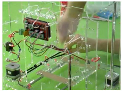
Thread the belt loop through a rectangular hole in the Inner Back and around the Y Motor pulley.
