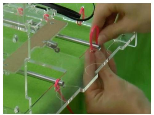
Insert the Y Assembly rods into slot in the bottom acrylic piece.
