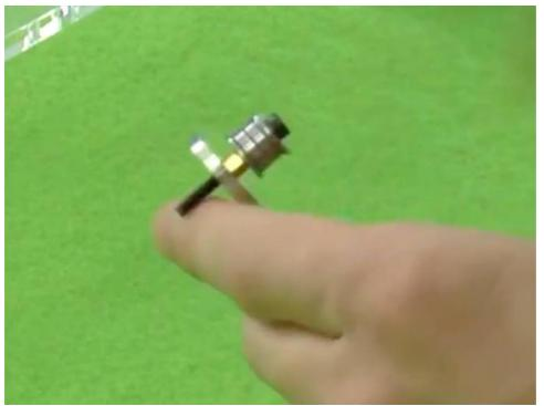
Put both two halves of the idler bearing onto the M3x25 bolt.
