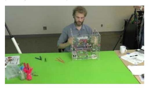
In this video, we incorporate Y assembly into the JellyBox frame. First, we'll install the Y Idler, and then the Y Bed Assembly.
