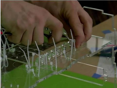
Align the wire comb with the corresponding annotations (ie. filament fan, heat block, etc.), and secure it with two zip ties.
