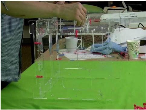
Insert 4" zip ties with the head on the outside (facing you) anywhere where there is a pair of holes 'connected' with an etching.
