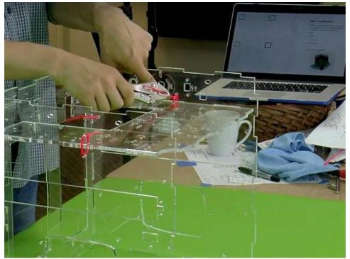
When the head of the zip tie touches the side you can't pull it tighter. Keep the head in the mid-air for the best results.
