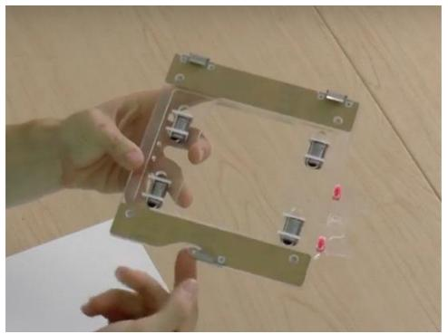
Make two loops out of 6" zip ties above and below the jelly jar. These loops will help correctly position the build plate. The heads of the zip ties need to be **on the bottom.**
