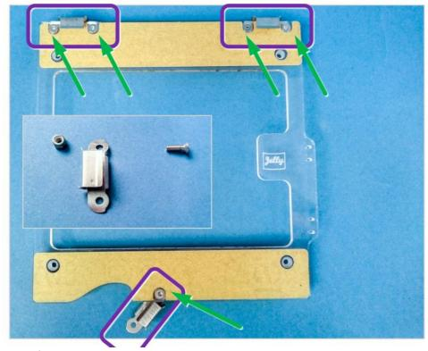
**In the front**, attach the one clip that is bent.
