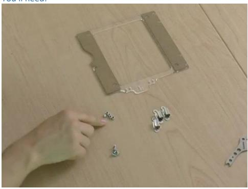
Top of Y-Assembly (with "Jelly" etching) Bed clips (3x) M3x8 flathead screws (5) Nylon lock nuts (5x)
