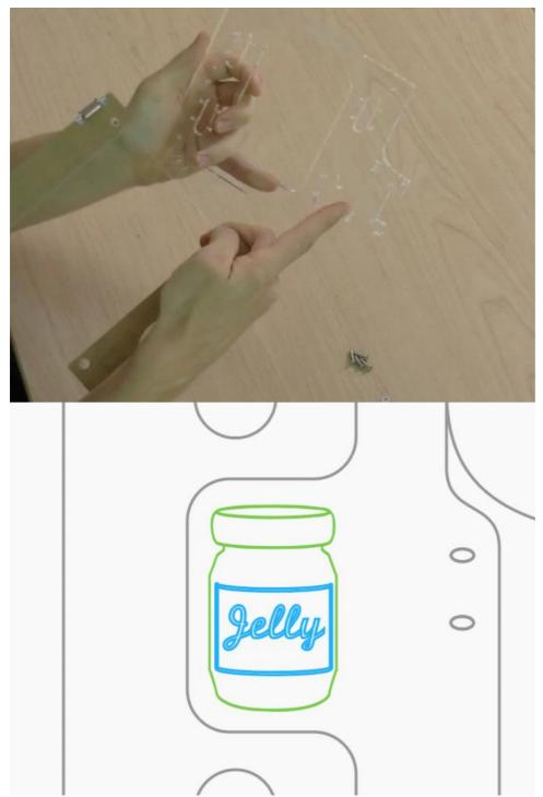
Sandwich the top and bottom acrylic piece so that the "Jelly" label lays on top of the outline of a jar.
