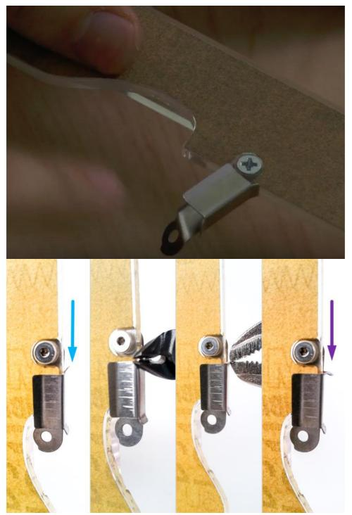
Bend a part of the front clip down along the diagonal line (shown in the drawing) with your vise grip.
