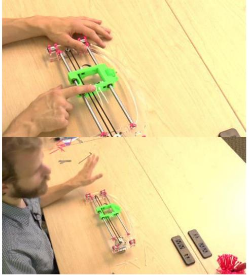
Loop in two small 4" zip ties around the belt through the X carriage on the motor facing side.
