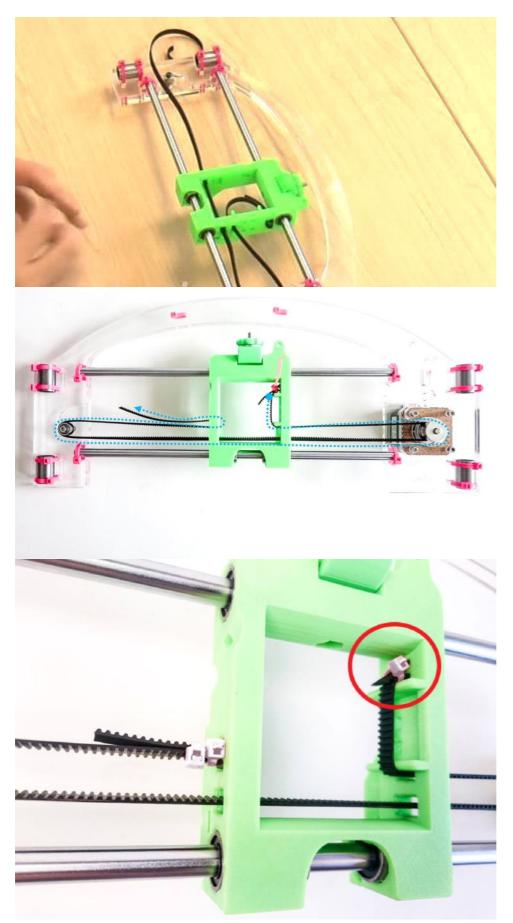
Thread the X Belt through the X carriage, around the X motor pulley, and around the X idler.
