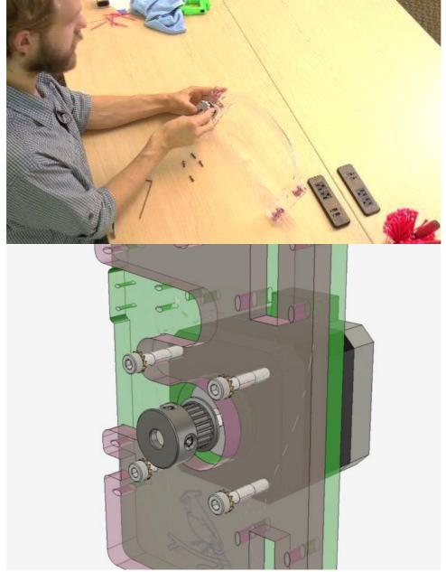
Follow the instructions etched on the X assembly, "X Motor adjoins right here to this side". The text is located just above the bird.
