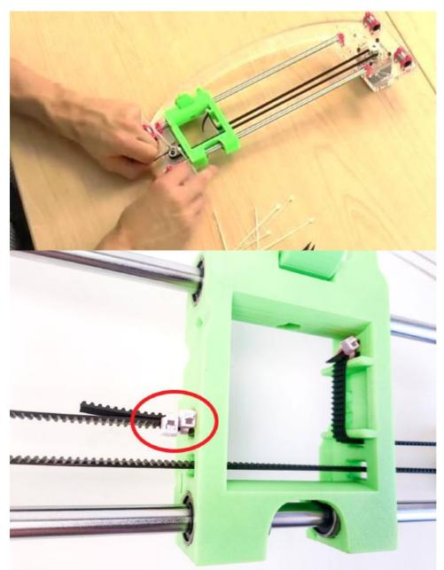
On the idler side, pull the belt tight and secure it with two 4" zip ties. (Good job for two. One pulls while the other one tightens zip ties.) Check: The belt should be slightly tight when you finish.
