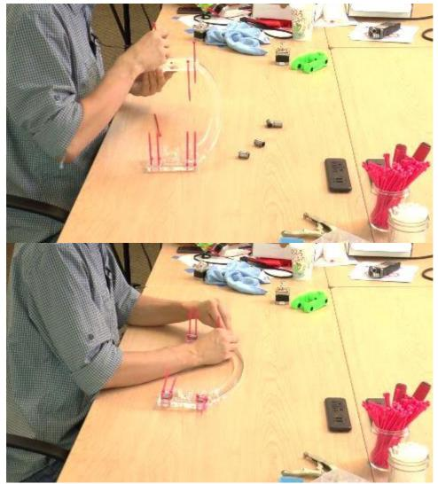
Thread in 8 zip ties through holes in the joined acrylic piece on both sidea of the assembly.
