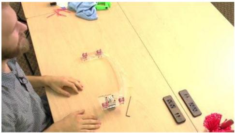
Turn the X assembly over with the X motor securely in place aligned properly and secure it to the assembly with the M3x16 bolts and serrated washers.
