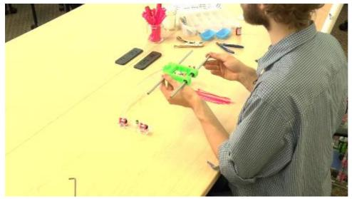
Slide two smooth rods through the X carriage bearings.
