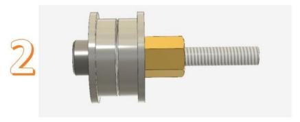
First, slide the two x idler bearings onto the M3x25 bolt and tighten them with 4mm hex spacer. (That's the **shorter of the two spacers**!) Tighten well.
