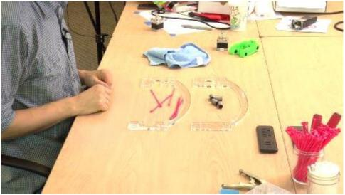
X assembly front and back acrylic pieces LM8UU linear bearings (4) 6" zip ties (8) Vise grip
