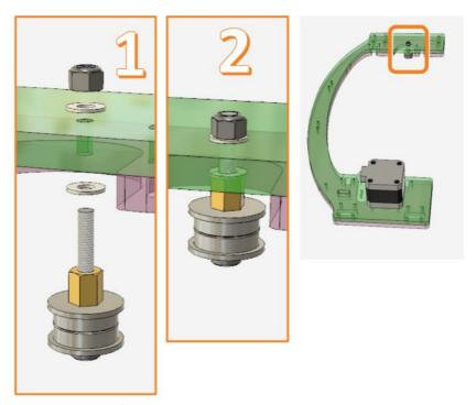
Tighten well and don't crack the acrylic.
