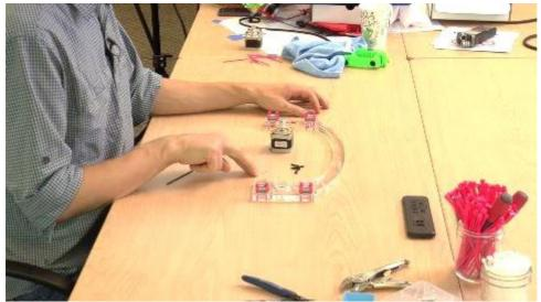
X assembly X motor M3x16 bolts (4) M3 serrated washers (4)
