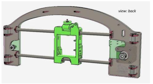
Check: the smooth side of the X Carriage must be facing the back - same side as motor pulley and idler.
