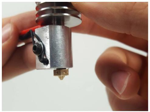
There should still be a small gap between the nozzle and the heatblock. The gap can be smaller than the one in the picture, but some gap must be there.
