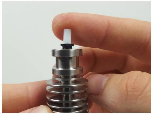
The PTFE should be sticking out on the top and not moving in any direction. The black collet should be all the way up.
