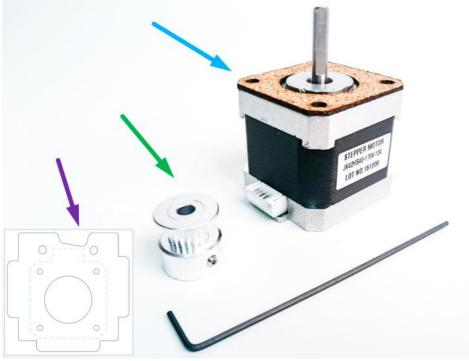
Y Bracket acrylic piece Y Motor (marked with a Y label) M3 hex key M3x12 bolts (4) M3 serrated washers (4)
