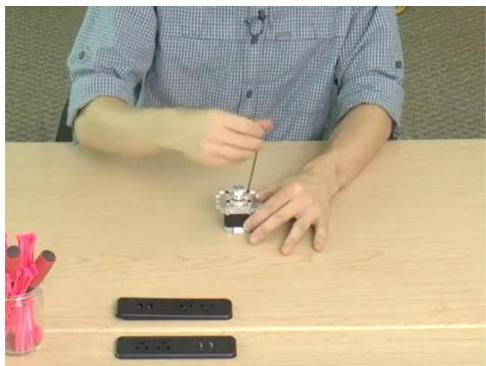
Tighten the bolts with the **short leg** of your M3 hex key. (To avoid overtightening. Good trick.)
