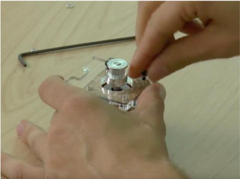
Finger-tighten the bolts into the 4 holes in the motor.
