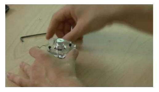
In this video, we install the Y motor onto the Y motor bracket.
