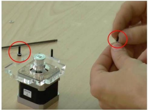
Place one serrated washer on each of the four bolts.
