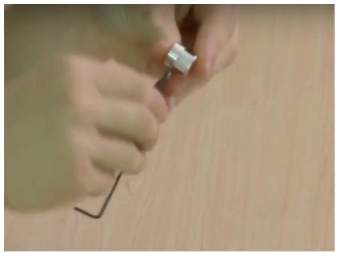
Re-insert the set screws into the pulley. Repeat procedure for both set screws.
