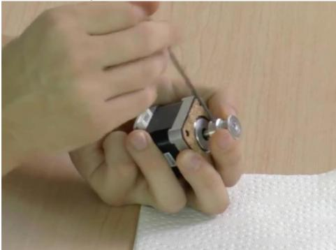
Slide the Y pulley onto the Y motor shaft.
