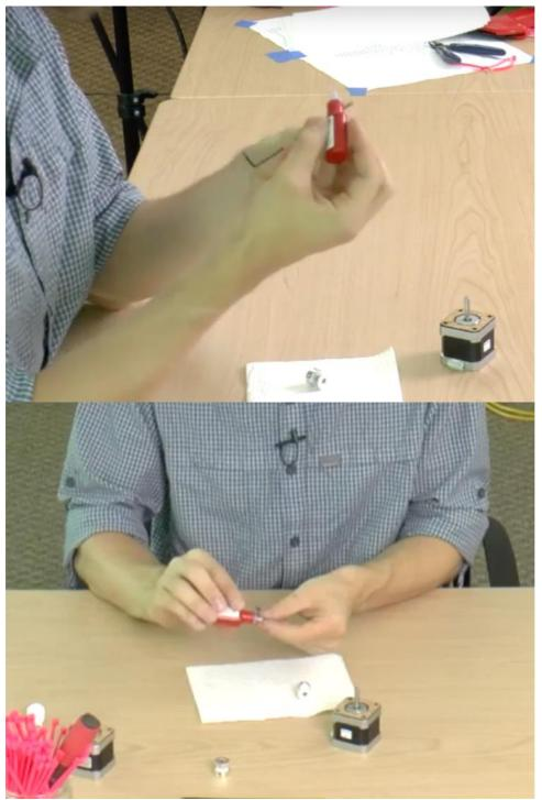
Put a single small drop of thread lock onto the set screw thread. Spread the thread lock into the thread.
