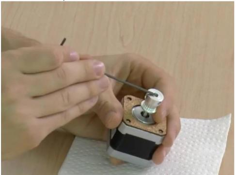
Slide the X pulley onto the Y motor shaft.
