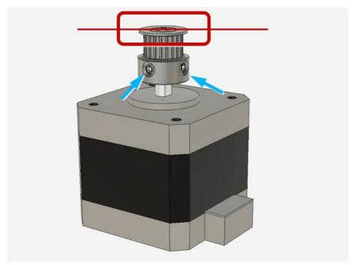
Align the top of the shaft with the top of the pulley.
