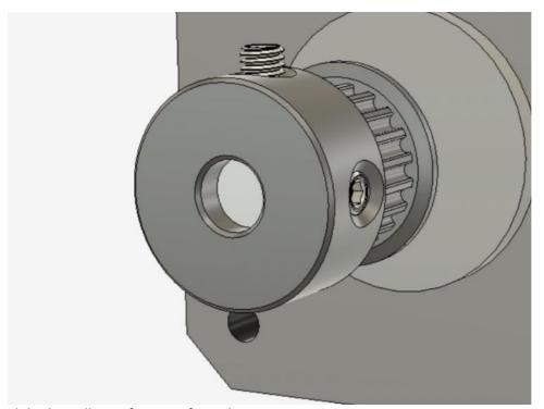
Slide the pulley as far away from the motor as you can. Yet the set screws should still fully grip the motor shaft.
