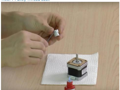
Take out two set screws out of a pulley using a hex key.
